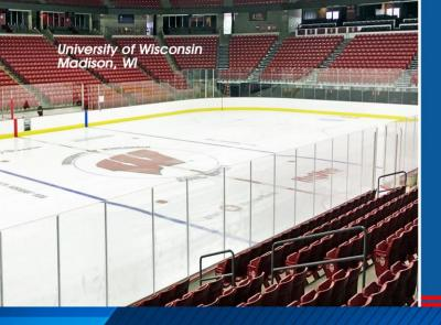
Our Legacy Elite™ aluminum dasher boards are a smart choice for professional, university, college, and community facilities that may require frequent changeovers. This system features a 6" welded aluminum framework that is 40% lighter than steel, designed with precision gate hardware, and enhanced player safety. Posted shielding comes in acrylic, tempered, or seamless glass; giving a clear unobstructed view. Made in the USA.
